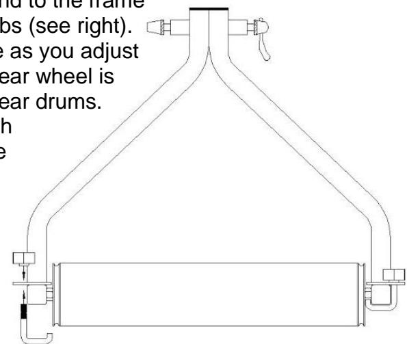
Remove your front wheel and assemble your bike to the skewer using the standard adjustment procedure for quick-release skewers.
