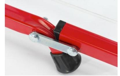
Adjust front drum by folding the frame to remove the tension on the belt, then removing the knobs on both sides of the drum. If one knob stays tight while the other one comes loose, screw the loose knob back onto the axle approximately 2-3 turns, then push the knob sideways slightly to put a slight bind onto the threads. Now loosen the other knob.
