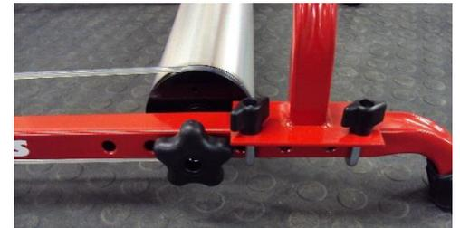
**In any case, the front roller drum should clear the fork stand when it is installed on the roller frame.**
